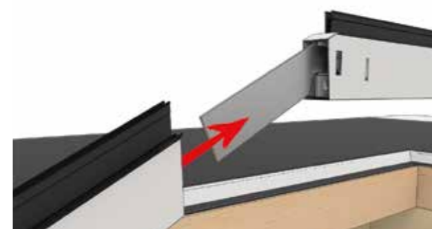
1 Slide central bell rafter over the factory-fitted bracket.
